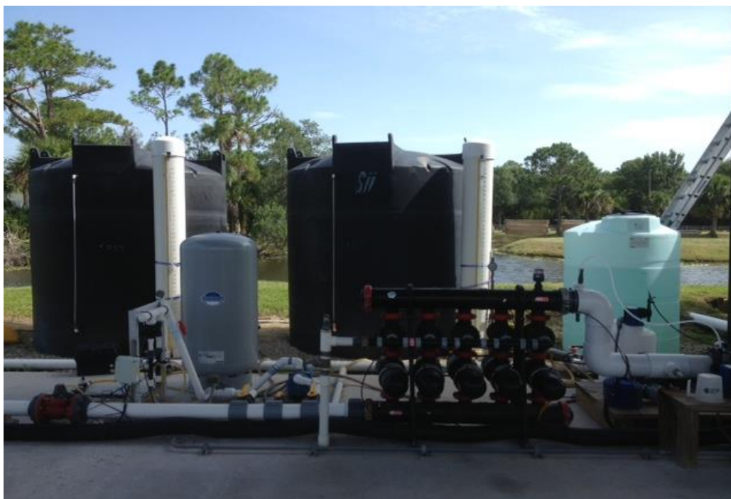
Figure 3-5. Blue/green fertilizer solution tank with fertilizer made to a specific concentration and then injected into irrigation water for greenhouse crop production.
